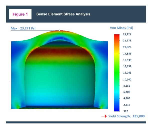
Von Mises Stresses on the sense element with 4,600 Psi applied. A max stress of 23,721 Psi is located on the top surface of the flexure. Deformation is exaggerated for clarity. Features that are non-critical to the analysis are not shown for proprietary reasons.
